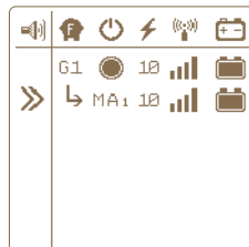
Overview screen with the subordinated monitor - to energizer G1
